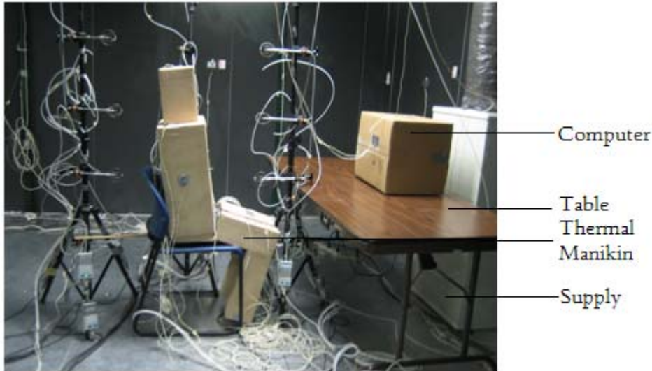
Figure 3.5 Configuration of environmental chamber in PDV experiments
