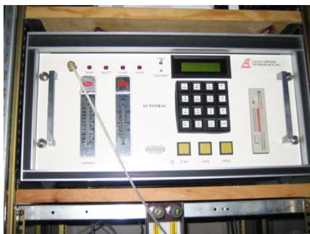
Figure 3.9 SF 6 collection and analysis system
